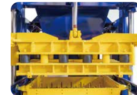
Double Oil Cylinder for Press Head, Special designed Synchronous Demolding Structure Ensure the very smooth molding and demolding during the machine working, make the machine very stable.
