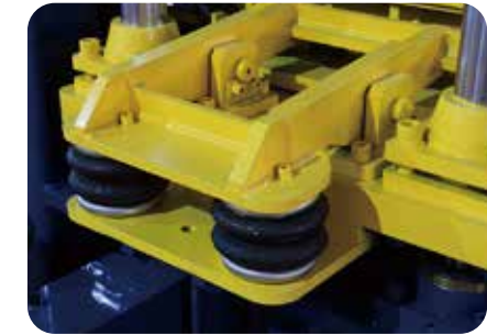
Air Bags for Mold Clamping Ensures that the mold is balanced and not easy to wear, also greatly reduce the molding changing time from 3 hours to 45mins.
