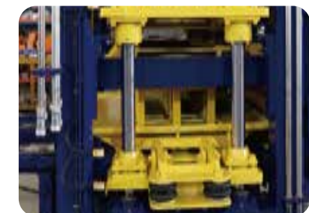
Special Designed Synchronization Device Ensure the same height of the concrete products
