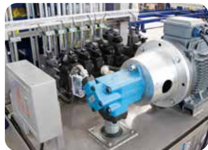
Hydraulic System Designed with Dual High Dynamic Proportional Valves and Counter Valve
