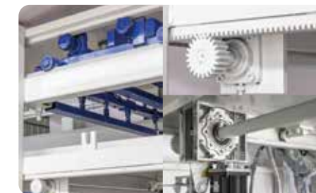
5. Use full set of Servo motors-controlled gear wheel and tooth row design for the block pushing, which is very stable, fast and accurate. Most other manufacturers use chains together with encoders to drive the block pushing, very low accuracy, non stable and the blocks are easily fell off during this process.
