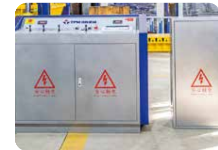
Siemens PLC Control System and Siemens Remote Control System Ensure the stability, reliability and easy maintenance of the circuit of the production line.
