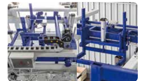
6. Special designed block protection device, to avoid blocks are fell off during the palletizing.
