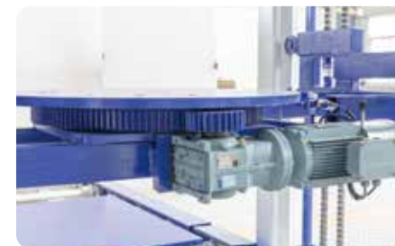
4. Our special designed - Gear rotating support structure, together with GuoMao new designed Reduer, no gap rotation is achieved, no shake during rotation, which guarantee the bricks/blocks are not dropped off during rotation.
