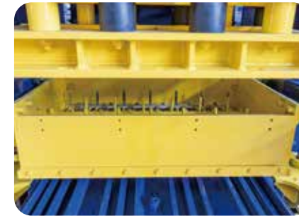
Double Swing arms Driven Feeder Car Equips with wear-resistant feeding rails, compulsory rotating mold filling, ensure the production speed and guarantee the high density of concrete products
