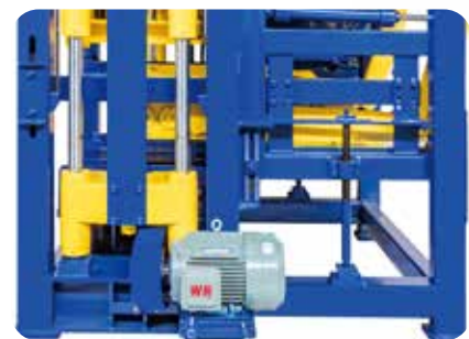
2x7.5kW Inverter Controlled Vibration Motors Controlled by double frequency inverters, the vibration force can be adjusted to ensure the quality of concrete products
