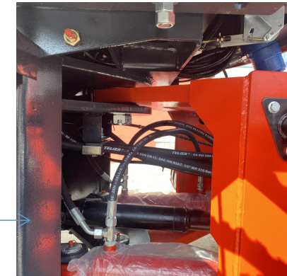
ANTICORROSION SPRAY PIPE
